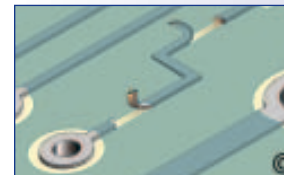
1. Remove damaged conductor.
