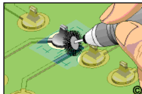
Figure 3: Rotary brushes are used to remove soft coatings or on contoured surfaces.
