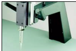
Figure 6: Bond the new land with a Bonding Iron or Circuit Bonding System.
