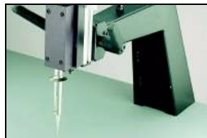
Figure 6: Bond the new pad with a Bonding Iron or Circuit Bonding System.
