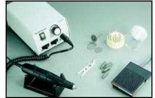
Figure 1: Drill out the hole using a Micro-Drill System or Mill Handle and Ball Mill.
