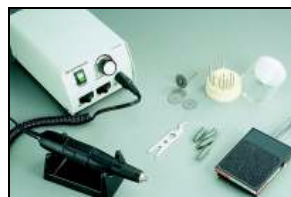
Figure 2: The Micro-Drill System is ideally suited for delicate circuit cuts.
