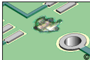
Figure 3: Epoxy can be used to repair damaged base board.
